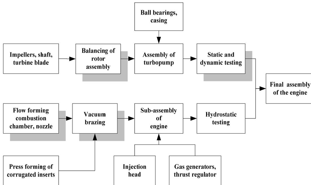
Figure II. Production flow chart for a liquid propellant propulsion system
