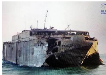
Figure 13.3 Impact point of ASM on Starboard Bow
