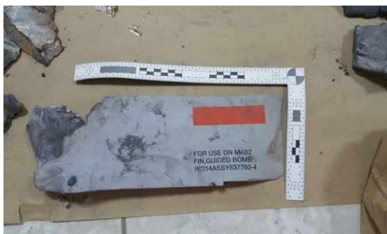
Figure 49.D.7 GBU-12 PAVEWAY II guidance unit Recovered and cleaned fin fragment
