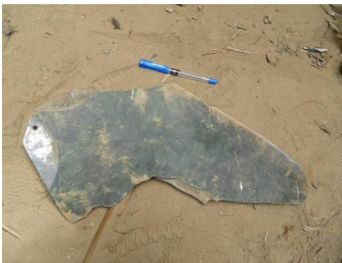
Figure 49.A.2 Rear fin from PAVEWAY terminal guidance unit 216
