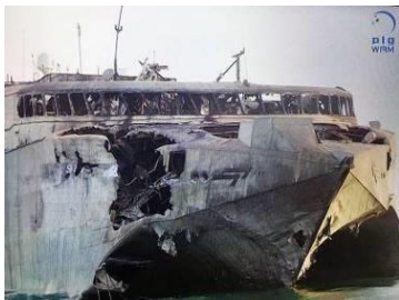
Figure 13.4 Exit point of ASM Port Midships
