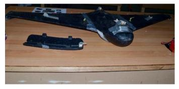
Figure V Qasef-1 loitering munition based on the Ababil-2/T
