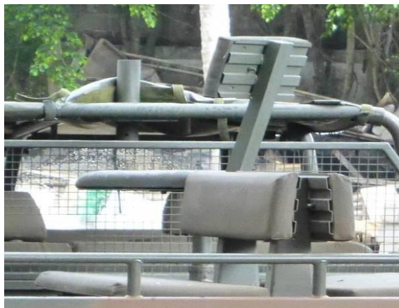
Gunner seat and mounting for a machinegun (12.7mm or 7.62mm) on the roof
