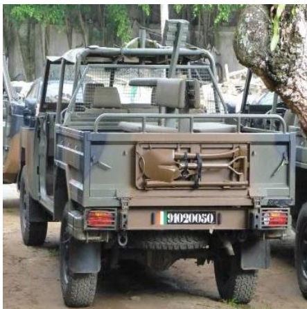
Gunner seat and mounting for a machinegun (12.7mm or 7.62mm) on the roof
