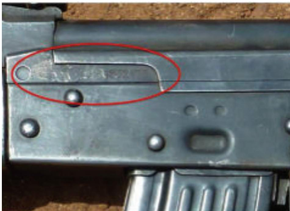
Note : As observed for samples A and B, serial numbers remain, but the manufacturer's marking has been erased.
