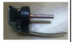
The detonator is red laquered at its interface to the fuze-head (Arges does not laquer outside)
