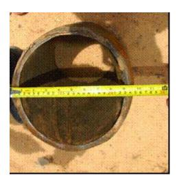
Photo 20 Circular face plate from bomb along with pieces of scrap metal packed inside in order to magnify potential casualties, Jebel Moon, 21 August 2008
