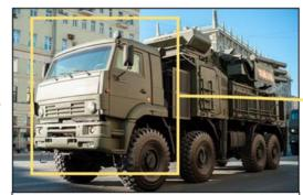
Production Pantsir S-1 on KaMAZ 6560 ground mobility platform. NOTE: Distinct driver cab differences: 1) sloping cab; 2) drivers steps; 3) front bumber; 4) window shapes; etc..
