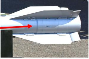
A. Imagery of missile remnant Note: Reduction in fuselage diameter (identifiable after "trumpeting" due to impact)
