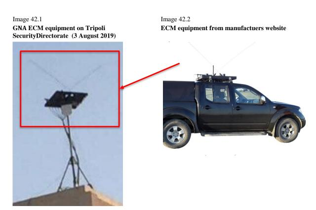
Note virtually identical angle and length of V-Pole antennae.
