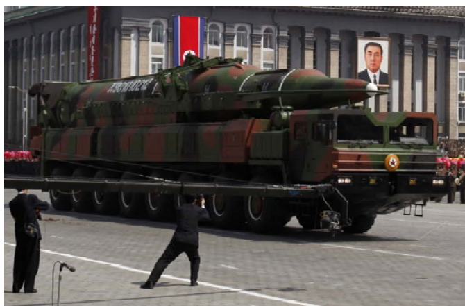
Figure V KN-08 missile on 8-axle transporter erector launcher
