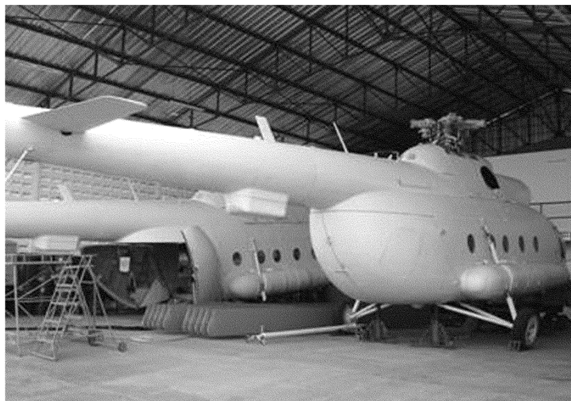
Photo 5: Mi-8T bodies being refurbished in Lomé
