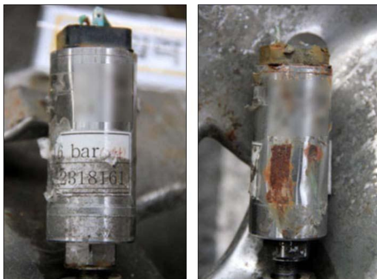
Figure IX Pressure transmitters found among the Unha-3 debris
