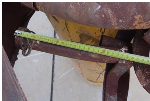
FIGURE 14: VISIBLE DAMAGE AND ADDITIONAL STRUCTURE ATTACHED TO ONE CYLINDER
