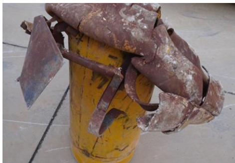
FIGURE 14: VISIBLE DAMAGE AND ADDITIONAL STRUCTURE ATTACHED TO ONE CYLINDER
